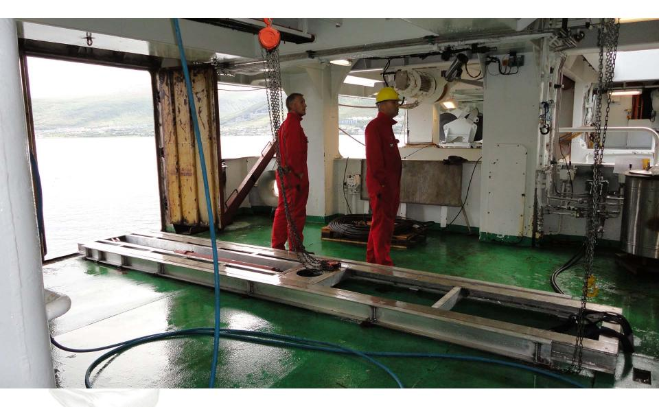
The base for the "stinger" is fixed on deck. The base can be moved for clearance to the door.
