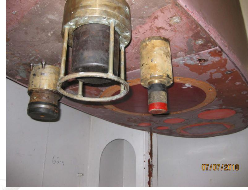
Hydrophones for commands and data communication installed in drop keel.
